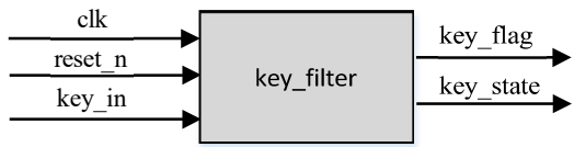
Figure 11-11 Key Debounce Module Interface
