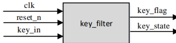
Figure 78: Key debounce module interface
