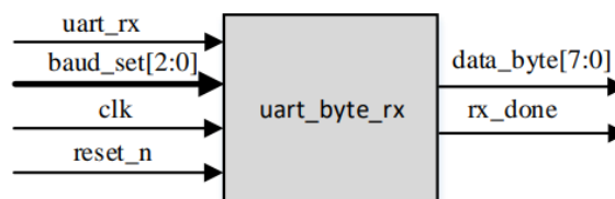
Figure 87: UART_RX receive module
